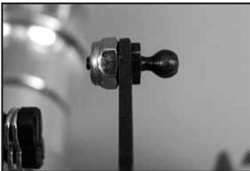
8. Install a 2-56 ball links (not included) to the throttle & choke control arms. Use a 2-56 lock nut to secure the ball links or use (2) 2-56 nuts and thread locker to secure the links. Once the links are secure, exercise the throttle and choke levers to ensure that no binding occurs.
